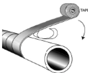
Fig 4. Diagram showing the correct application of tape.
