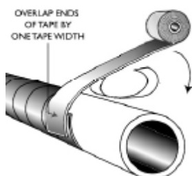
Fig 4. Diagram showing the correct application of tape.
