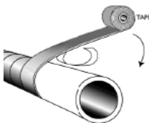
Fig 4. Diagram showing the correct application of tape.
