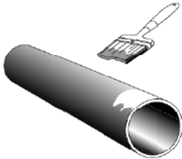
Fig 1. Priming pipes: Apply ECOTAPE P29 PRIMER to entire area to be protected with tape.
